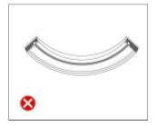
Face to the side surface, (as the picture shows) Do not bend downward to damage the strip
