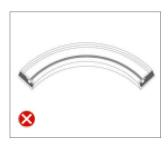
Face to the side surface, (as the picture, shows) Do not bend downward to damage the strip
